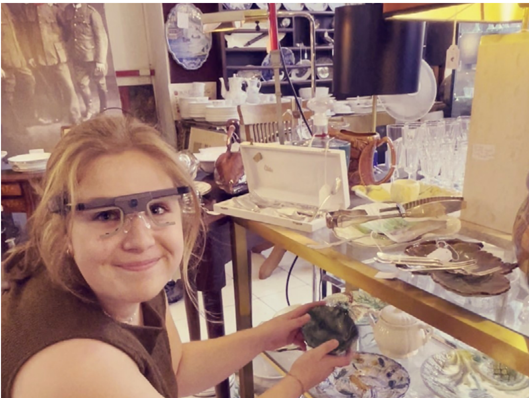
The participants wear glasses equipped with a minicamera and an eye-tracking device that record a first-person video.
